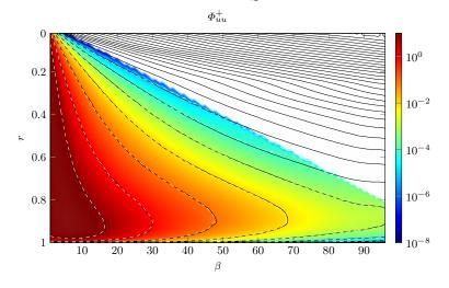
Figure 4: Spectral energy density  $\Phi_{tut}^+$  of the axial velocity fluctuations in the  $r - \beta$  plane. Black contour lines are from the simulation with constant azimuthal resolution, and the colormap with white dashed contours is from the the simulation where the number of azimuthal modes varies with *r*. Contour levels start from 10<sup>0</sup>, spaced by one order of magnitude.
