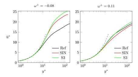
Figure 7: Mean streamwise velocity profile for two cases with drag reduction  $(\omega^+ = -0.08, \text{ left})$  and drag increase or minimal drag reduction  $(\omega^+ = 0.11, \text{ right})$ . Cases SIN and S3 are compared to the uncontrolled flow.
