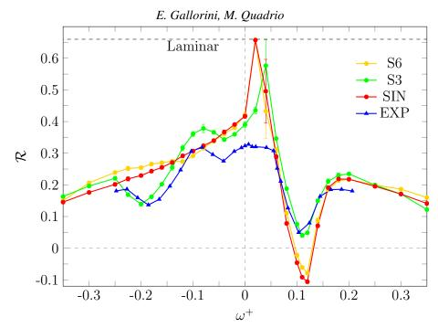
Figure 5: Drag reduction rate  $\mathcal{R}$  computed with DNS against experimental measurements from ABBCQ (blue triangles, blue line). The plot shows the laminar limit (upper dashed line), and quantifies with bars the error deriving from the finite averaging time (see text).
