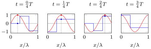
Figure 10: SIN (red line) and S3 (blue line) wall forcing along one wavelength, at four different times during the period T. At each time, the dots mark the position at which SIN is maximum.
