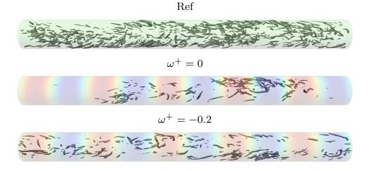
Figure 14: Instantaneous snapshot of the reference and sinusoidally forced pipe flow, with parameters yielding drag reduction above ( $\omega^+ = 0$ ) and below ( $\omega^+ = -0.2$ ) the apparent experimental threshold for  $\mathcal{R}$ . The background colormap (from blu to red) encodes the azimuthal velocity of the wall; the grey isosurfaces are drawn for  $\lambda_2^+ = -0.03$ .
