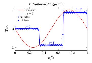
Figure 2: Schematics of the spatial waveform for the control: the red line is the sinusoidal wave, and the blue line is its discrete approximation by three segments per period, i.e., s = 3. The corresponding representation after the Fourier transform without (empty symbols) and with (filled symbols) spatial filtering is also depicted.
