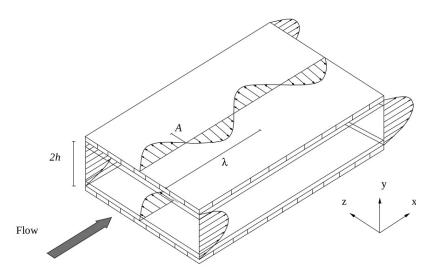
FIG. 1. Sketch of plane channel with the chosen reference system. The two channel walls are separated by a distance 2h; a stationary wall forcing is applied at both walls, and is characterized by its wavelength  $\lambda$  and maximum velocity amplitude A.
