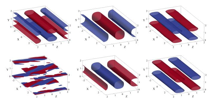
FIG. 7. Optimal initial condition computed for Re = 2000,  $\kappa = 1$  and  $\beta = 1.5$ : unforced flow at A = 0 (top) and forced flow at A = 1 (bottom). For each velocity component (u, v, w) from left to right) isosurfaces at  $\pm 60\%$  of their respective maxima are visualized. After normalizing the perturbation to unit maximum amplitude, the u, v, w components of the maximum are 0.11, 2.68, 3.79 for A = 0, and 0.74, 2.63, 3.79 for the A = 1 case.
