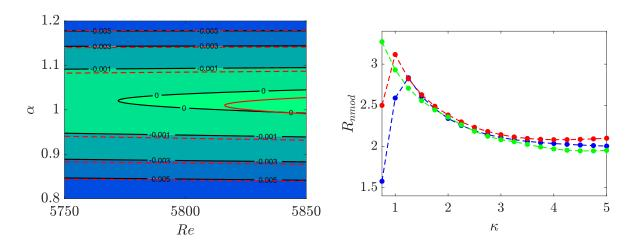
FIG. 9. Modal and non-modal stability characteristics computed by taking  $\beta$  as a free parameter to select the worst case. Left: neutral stability curves for the unforced flow (contour plot and black lines) and the forced flow (red lines) for A=1 and  $\kappa=3$ . Right: dependence of  $R_{nmod}$  on  $\kappa$  at A=1 and Re=500 (blue), Re=1000 (red) and Re=2000 (green).
