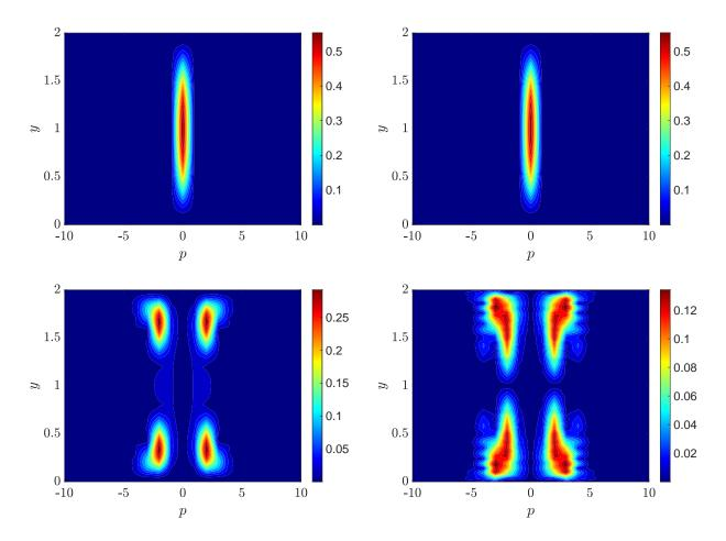
FIG. 11. Optimal initial condition, at Re=1000 for v (left) and  $\eta$  (right) as a function of the y coordinate and the p-th wavenumber of the modal expansions,  $-M \le p \le M$ . Contours describe the absolute value of the optimal initial condition. Top: example of optimal input centered around p=0, with  $\kappa=1.5$ , A=0.3 and  $\beta=0.5$ . Bottom: example of optimal input peaking at  $\alpha \sim \pm \kappa^{-1}$  with  $\kappa=1$ , A=0.6 and  $\beta=0.3$ .
