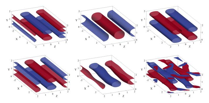
FIG. 8. Evolution of the optimal initial condition at the time of maximum energy growth, computed for Re = 2000,  $\kappa = 1$  and  $\beta = 1.5$ : unforced flow at A = 0 (top) and forced flow at A = 1 (bottom). For each velocity component (u, v, w) from left to right) isosurfaces at  $\pm 60\%$  of their respective maxima are visualized. The u, v, w-components change by a factor of 481, 0.47, 0.40 for A = 0, and by a factor of 44, 0.51, 0.46 for A = 1 with respect to the initial condition.
