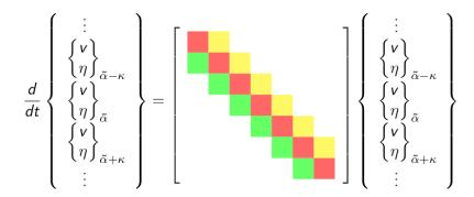
FIG. 2. Graphical representation of the system  $\dot{\mathbf{q}} = \mathbf{A}_s \mathbf{q}$ . The matrix is block-tridiagonal with block size  $M \times M$ . The red blocks on the diagonal correspond to the classic OSS matrices for each streamwise wavenumber, whereas the adjacent green and yellow blocks describe interactions with contiguous streamwise wavenumbers.
