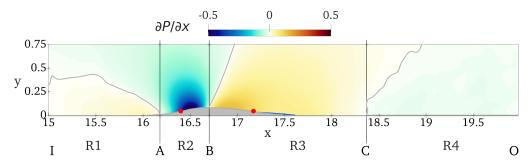
Figure 4: Mean streamwise pressure gradient  $\partial P/\partial x$ . The contour line is for  $\partial P/\partial x=0$ . The barely visible reverse flow region is shown via the U=0 line in blue. Red circles indicate the two inflection points.
