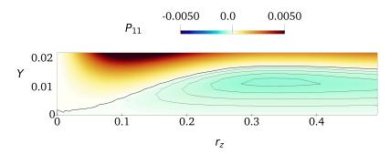
Figure 12: Zoom of the production term  $P_{11}$  in the recirculating bubble at X = 17.75. The black thick line is for  $P_{11} = 0$ . The black thin lines indicate isovalues of  $P_{11}$ , with an increase of 0.0002.
