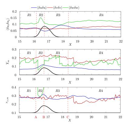
Figure 6: Streamwise evolution of the intensity and the  $(Y,r_z)$  location of the maxima of the diagonal components of the structure function tensor. The intensity of  $\langle \delta v \delta v \rangle$  and  $\langle \delta w \delta w \rangle$  in the top panel is multiplied by a factor of 10 for visualisation. The black line shows the bump (arbitrary vertical scale). Regions identified by the dashed lines are defined in Figure 4.
