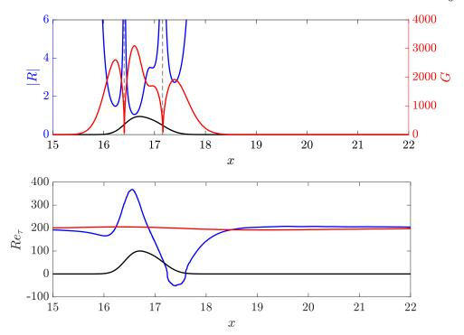
Figure 2: Top: streamwise evolution of the (absolute value of the) curvature radius R (blue line), with dashed lines indicating vertical asymptotes; the red line shows for the streamwise evolution of the Görtler number, defined in the text. Bottom: streamwise evolution of  $Re_{\tau}$  on the bottom (blue) and top (red) walls. In both plots, the bump is drawn with arbitrary vertical scale.
