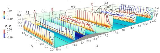
Figure 15: Colormap of the complete source term  $\xi$  on selected planes (where the black contour line indicates the level  $\xi = 0$ ), and field lines of the flux vector  $\Phi'$ , coloured by the flux divergence.
