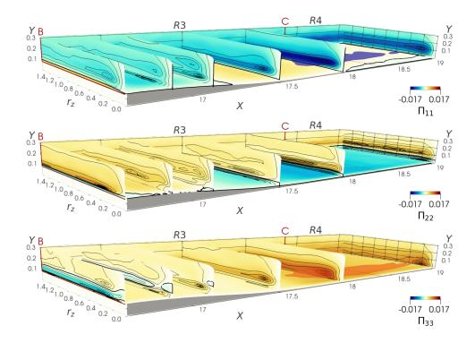
Figure 13: Pressure–strain terms  $\Pi_{11}$  (top),  $\Pi_{22}$  (center) and  $\Pi_{33}$  (bottom). See caption of figure 10 for contour lines and isosurfaces.
