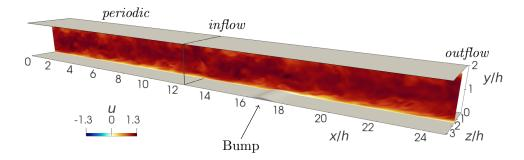
Figure 1: Sketch of the computational domain and the reference frame. The portion with  $x/h < 4\pi$  corresponds to a periodic plane channel flow; the peak of the small bump is at  $x/h \approx 16.7$ . An instantaneous snapshot of the streamwise velocity field u is plotted on a streamwise-parallel plane; flow is from left to right.
