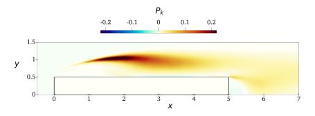
Figure 8: Map of the production term  $P_k$  of the turbulent kinetic energy for the sharp configuration.
