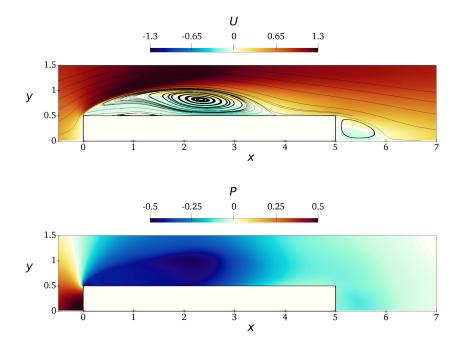
Figure 2: Mean flow. Top: streamlines and color contour for the mean streamwise velocity component U. Bottom: mean pressure P.
