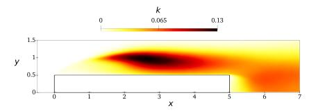
Figure 6: Map of the turbulent kinetic energy for the sharp configuration.
