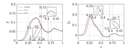
Figure 13: Evolution of k (left) and  $\xi_k$  (right) over the mean streamline originating at (x,y)=(0,0.5) shown in figure 4 as a function of the normalised curvilinear coordinate s. The left vertical dashed line marks the reattachment point, and the right dashed line marks the TE.
