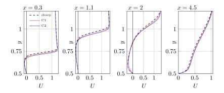
Figure 5: Vertical profiles of the streamwise component of the mean velocity U at four different stations over the cylinder side.
