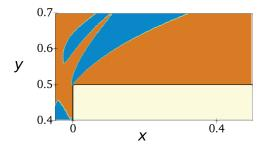
Figure 16: Sign of the change  $\delta(dy_s/dx)$  in the local slope of mean streamlines. Blue: negative change; orange: positive change.
