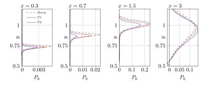
Figure 9: Vertical profiles of  $P_k$  at four different station over the cylinder side as in figure 7.
