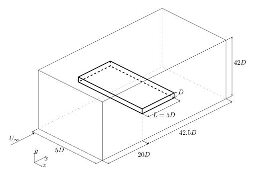
Figure 1: Sketch of the computational domain for the BARC flow, with the reference system.
