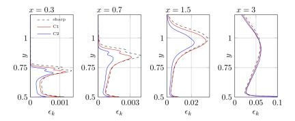
Figure 11: Vertical profiles of the dissipation rate of the turbulent kinetic energy at four different stations over the cylinder side.
