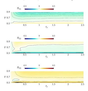
FIGURE 12. Two-dimensional view of the pressure-strain terms, in the plane X=4. Panels as in figure 10.
