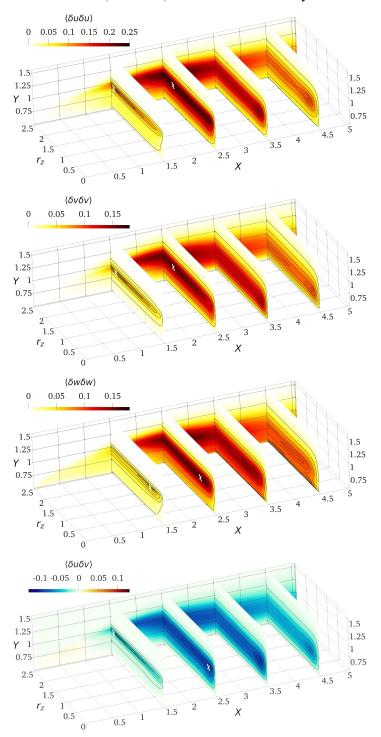
FIGURE 4. Components of the structure function tensor plotted in the space  $(X,Y,r_z)$  over the cylinder side. Contours in the planes X=1.5,2.5,3.5,4.5 are for the 99%, 95%, 90%, 75%, 50% and 20% of the in-plane maximum. White crosses are used to identify local maxima when not easily visible.
