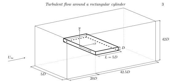
FIGURE 1. Sketch of the geometry, computational domain and reference system. The reference length is the body height D.
