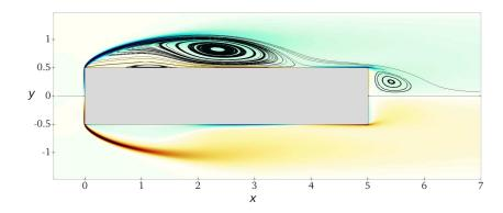
FIGURE 2. Mean streamlines (top half only) plotted over a colour contour of the mean spanwise vorticity  $\Omega_z$  (blue/red indicates negative/positive values in the range  $-20 \le \Omega_z \le 20$ ).
