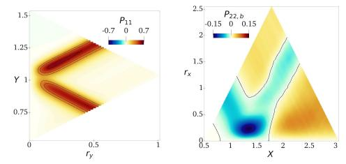
FIGURE 9. Production terms for  $\langle \delta u \delta u \rangle$  and  $\langle \delta v \delta v \rangle$  associated with the KH rolls. Left:  $P_{11}$  in the  $(Y, r_y)$  space with  $r_x = r_z = 0$ , X = 1.5 and  $0.5 \le Y \le 1.55$ . Right:  $P_{22}$  in the  $(X, r_x)$  space with  $r_y = r_z = 0$ , Y = 0.99 and  $0.5 \le X \le 3$ .
