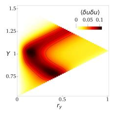
FIGURE 7.  $\langle \delta u \delta u \rangle$  in the  $(Y, r_y)$  space with  $r_x = r_z = 0$ , X = 1.5 and  $0.5 \le Y \le 1.55$ .
