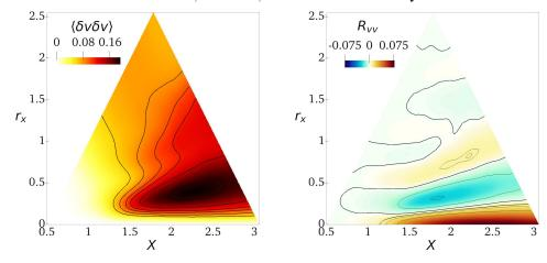
FIGURE 6.  $\langle \delta v \delta v \rangle$  (left) and  $R_{vv}$  (right) in the  $(X, r_x)$  space with  $r_y = r_z = 0$ , Y = 0.99 and  $0.5 \le X \le 3$ .
