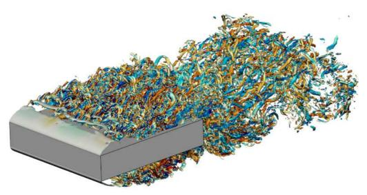
FIGURE 3. Instantaneous snapshot of the BARC flow: perspective view of the isosurfaces at  $\lambda_2 = -5$ . Color depicts streamwise vorticity  $\omega_x$ , with the blue-to-red colormap ranging in  $-10 \le \omega_x \le 10$ .
