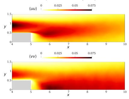
FIGURE 16. Maps of the  $\langle uu \rangle$  (top) and  $\langle vv \rangle$  (bottom) components of the Reynolds stresses in the x-y plane, with focus on the near wake.
