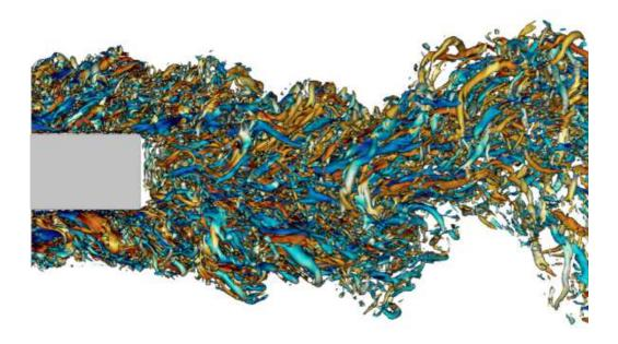
FIGURE 15. Instantaneous snapshot of the BARC flow: lateral view of the isosurfaces at  $\lambda_2 = -5$ , with zoom into the near-wake region. Colour depicts streamwise vorticity  $\omega_x$ , with the blue-to-red colormap ranging in  $-10 \le \omega_x \le 10$ . The vertical size D of the cylinder can be used as reference to identify the vertical and streamwise length scales of the near wake.
