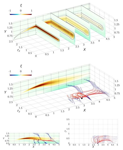
FIGURE 14. Field lines of the reduced fluxes for  $\langle \delta q^2 \rangle$  in the  $r_x = r_y = 0$  space. The top panel is for the source term  $\xi$ . In the central panel the colourmap on the  $r_z = 2.5$  plane is for  $\xi$  and the lines are coloured with the divergence of the reduced flux vector  $\nabla \cdot \hat{\Phi}$ : red/blue indicates positive/negative  $\nabla \cdot \hat{\Phi}$ . The lower panels are bottom and side views of the central one.
