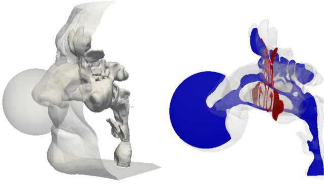
Fig. 2. Left: the whole computational domain, made by the inner airways plus the outer spherical volume. Right: sagittal (blue) and coronal (red) sections, showing the volume mesh for the finest mesh employed in this work, made by approximately 25 M cells. (For interpretation of the references to color in this figure legend, the reader is referred to the Web version of this article.)
