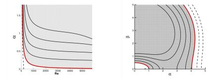
Contours of  $T(\alpha, \beta, Re) = \lambda_{max}(B^{\perp}(A + A^{H})B^{\perp H})$
