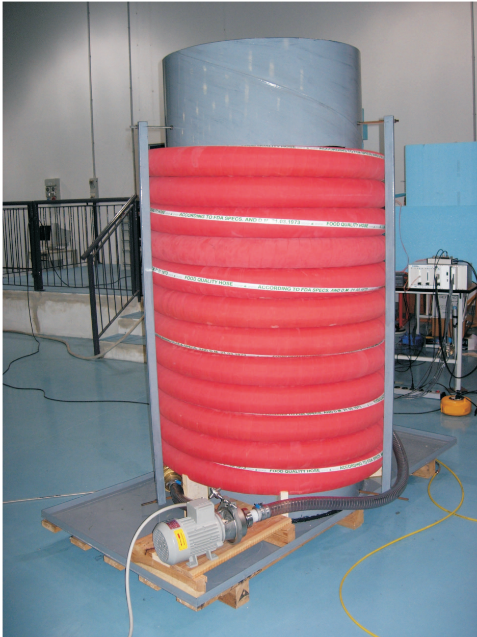
Figure 3.6: The helical pipe system.
