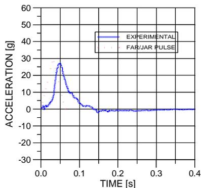
Fig. 14 – (60° case Poli) sled acceleration
