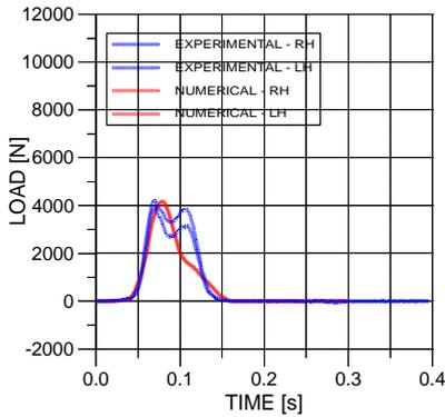
Fig. 5 – (0° case TNO) LH and RH shoulder belt loads
