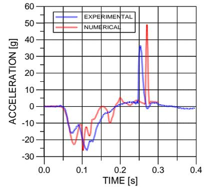
Fig. 7 – (0° case TNO) head front acceleration
