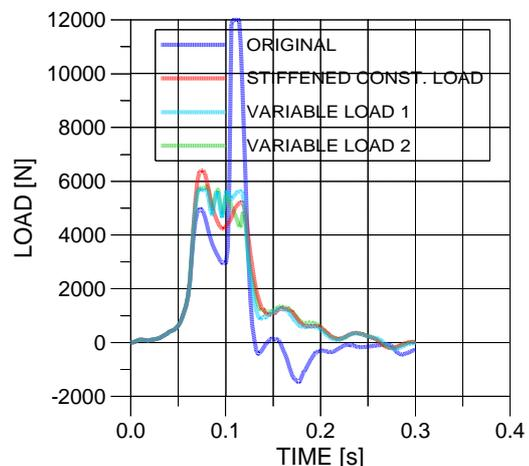
Fig. 21 – Dummy lumbar spine load
