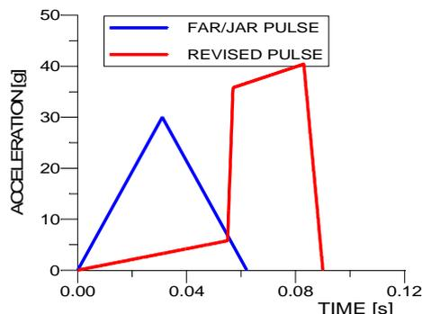
Fig. 3 – Test set-up (SIEMENS Laboratories), original and revised acceleration pulse
