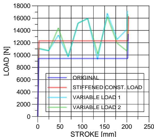
Fig. 20 – Energy absorber load profiles (dynamic)
