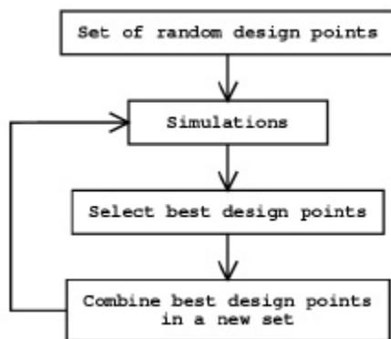
Fig. 22 – Flow diagram for the genetic algorithm
