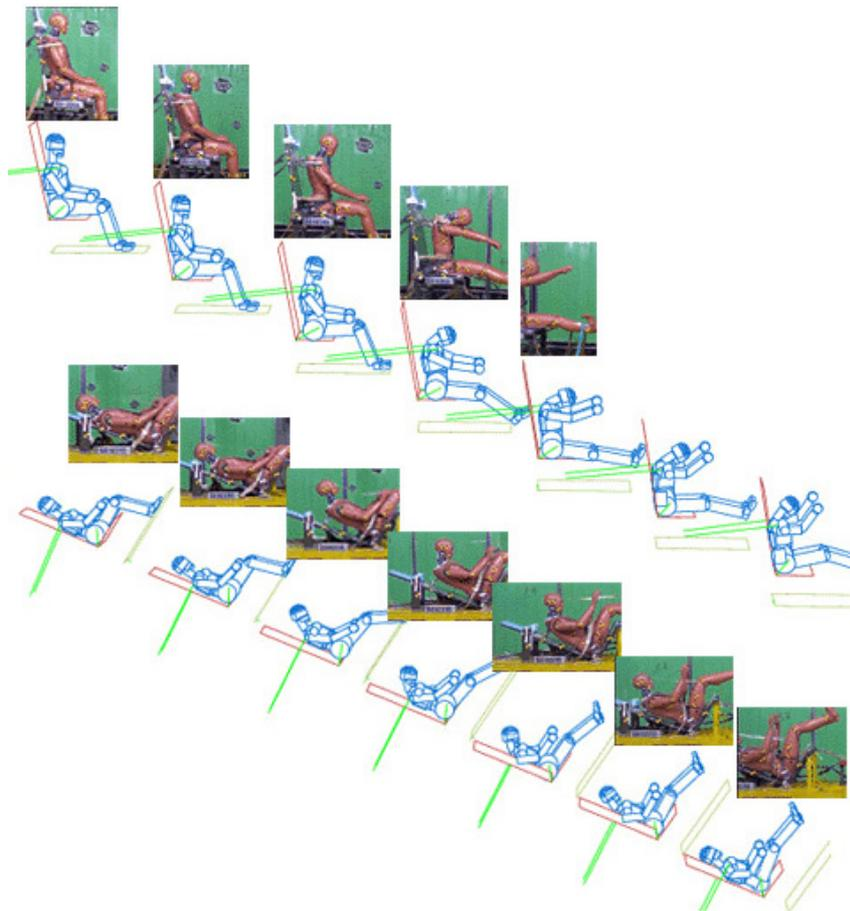
Fig. 4 – VEDYAC simulation of  $0^\circ$  and  $60^\circ$  TNO dynamic tests
