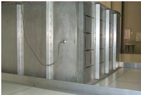
Fig. 6 - Test equipment: right side pressure transducer.
