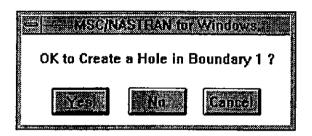
In the OK to Create a Hole in Boundary 1 box, choose Yes, and then select curve 9 (position the cursor over curve label 9 and click the mouse). Then choose OK to define the hole as curve 9. The box now asks, "OK to Create another Hole in Boundary 1?" and you choose No, since there is only one hole in this example.
