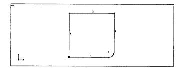
Now, change Curve1 to 2 and Curve2 to 3, and change X to 3 and Y to 3, to create a filleted corner between curves 2 and 3; choose OK to apply the fillet.
