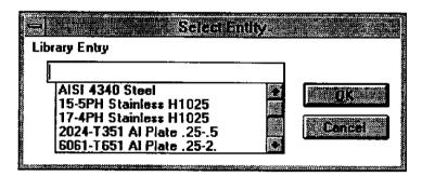
Select AISI 4340 Steel, choose OK, and note that the isotropic material properties are entered. Note that the Density is mass density, which is in units of lb-sec<sup>2</sup>/in.<sup>4</sup> for English units. Note, too, that the material ID is 1.
