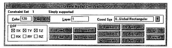
Select Pinned to define pinned supports, then choose **OK**. Pinned supports are applied to grid points 1 through 40 (the outer edge).
