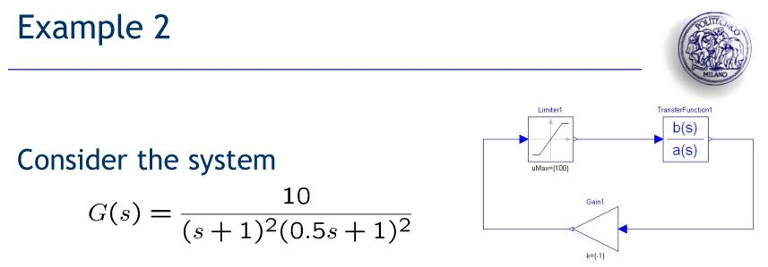
under feedback with a saturation of unit amplitude.
