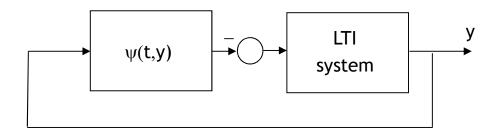
Frequently the linear part of the system is known and the problem is to study the effect that inserting a nonlinearity in the loop might have on the system's response.
