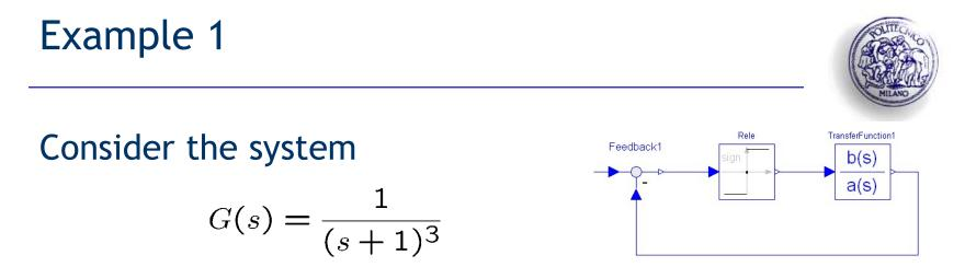
under feedback with a relay of unit amplitude.
