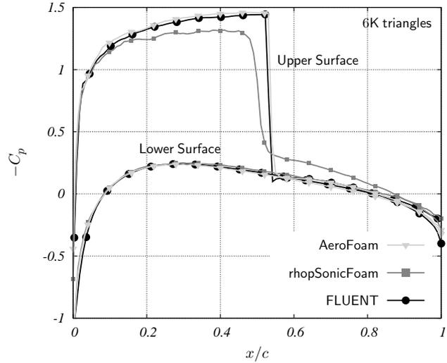
Figure 1: Transonic flow around the NACA 0012 airfoil at  $M_\infty = 0.75$  and  $\alpha = 4.00^\circ$  computed with AeroFoam. On the left the isolines of the pressure coefficient  $C_p$  are shown. On the right the distribution of the pressure coefficient  $C_p$  along the airfoil chord  $c$  computed with AeroFoam ( $\nabla$ ) is compared with rhoPsonicFoam ( $\blacksquare$ ) and FLUENT ( $\bullet$ ) results.
