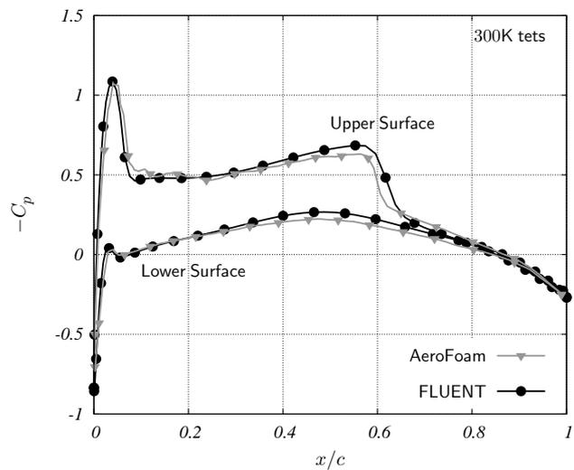
Figure 2: Steady-state transonic flow around the ONERA M6 wing at  $M_\infty = 0.84$  and  $\alpha = 3.06^\circ$  computed with AeroFoam. On the left the isolines of the thermodynamic pressure  $P$  on the wing and the symmetry plane are shown. The  $\lambda$ -shaped shock wave is accurately resolved. On the right the distribution of the pressure coefficient  $C_p$  at the wing span station  $y/b = 0.2$  computed with AeroFoam ( $\nabla$ ) is compared with FLUENT ( $\bullet$ ) results.
